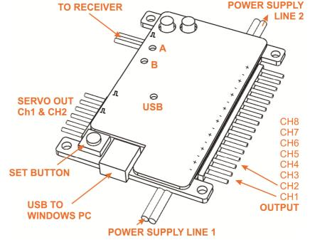
controller can be operated from USB without receiver but does not get live feedback from the receiver system. During normal operation, the complete USB electronic is inactive and does not interfere with the remote control.
